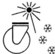
Overload through thermal effects
